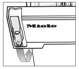
■ To clean the lint trap, remove the tool from behind the detergent dispenser drawer.
